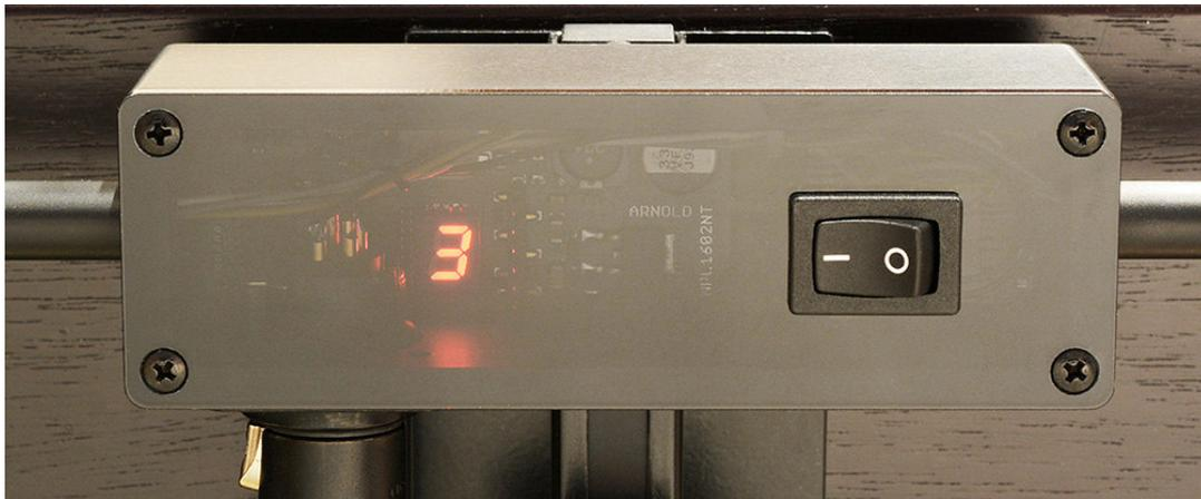
Now put the operating mode to a DMX mode or the Stand-Alone Mode. See Section 2.5.2 et sqq.. The number of the light goes out. In the DC MODE appears a small red dot in the light that indicates this mode.
