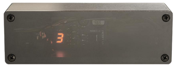
Electronic housing model NT (digital) (with 7-segment address display and IR sensor, DMX controllable with power supply SPY 600 NT)
